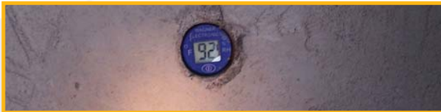
Above: Wagner RH probe installed in a slab Below: Moisture content in slab between Oct 07 and Jan 08
